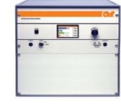
The Model 250S1G6 is a solid-state, Class A design, self-contained, aircooled, broadband power amplifier designed for applications where instantaneous bandwidth, high gain and linearity are required. It will provide a minimum of 250 W across its operating bandwidth. Protection from input overdrive beyond 0 dBm is provided as well as protection from various failure conditions including over-temperature and power supply faults.
